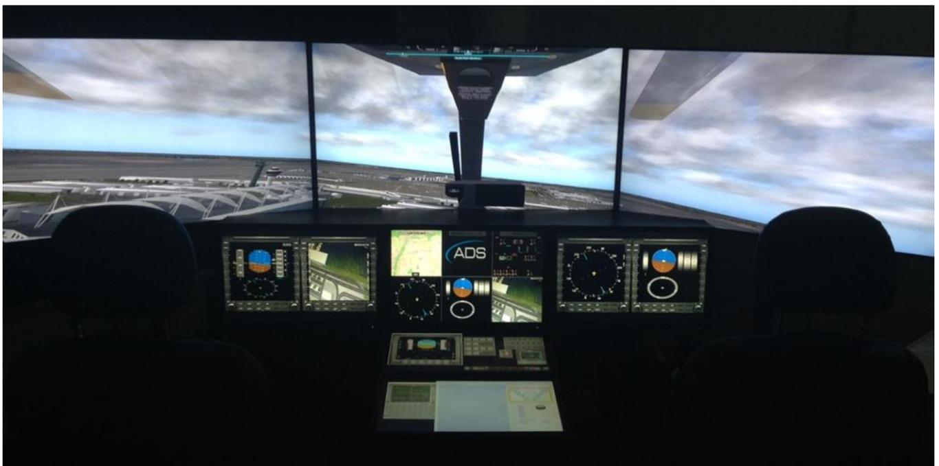
As older generation flight crew retire to be replaced by their younger counterparts, the tendency to accept the introduction of these new human machine interaction (HMI) concepts has increased. As such, avionics suppliers are now able to produce more flexible display designs allowing de-cluttering of the information presented to the aircrew. It is now possible to restrict the level of information density presented within the cockpit thus allowing the flight crew to focus on their current tasks.
