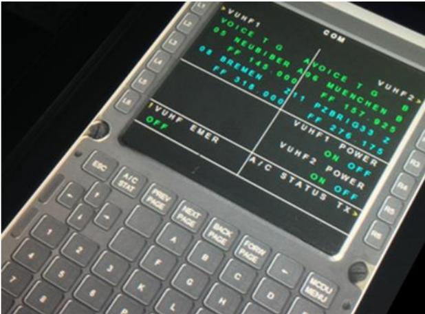
**Control & Display Unit Application and Page generation Tool compliant to ARINC 661 and ARINC 739**
